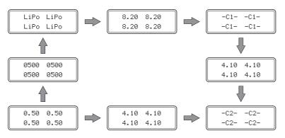
battery type -total voltage -1st cell voltage--2nd cell voltage-charging current- battery capacity of each port circularly.
